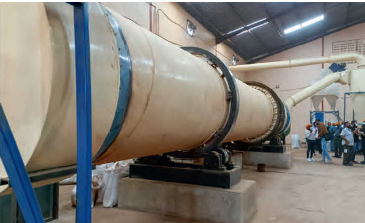
The direct-fired co-current rotary drum dryer.
