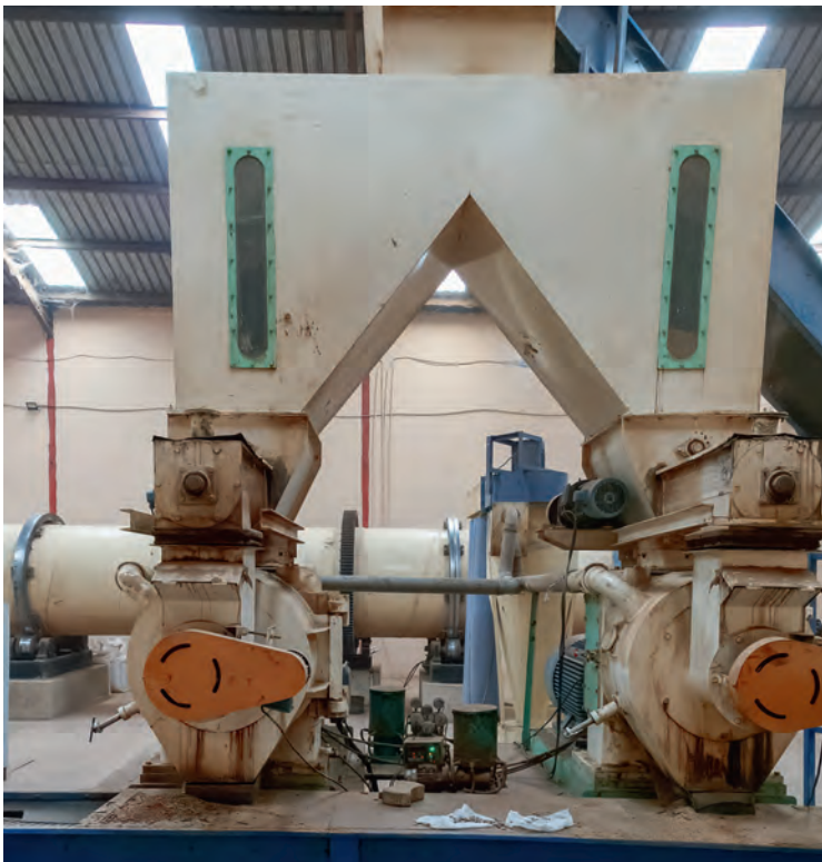
A single hopper feeds a set of twin pelletizers.
