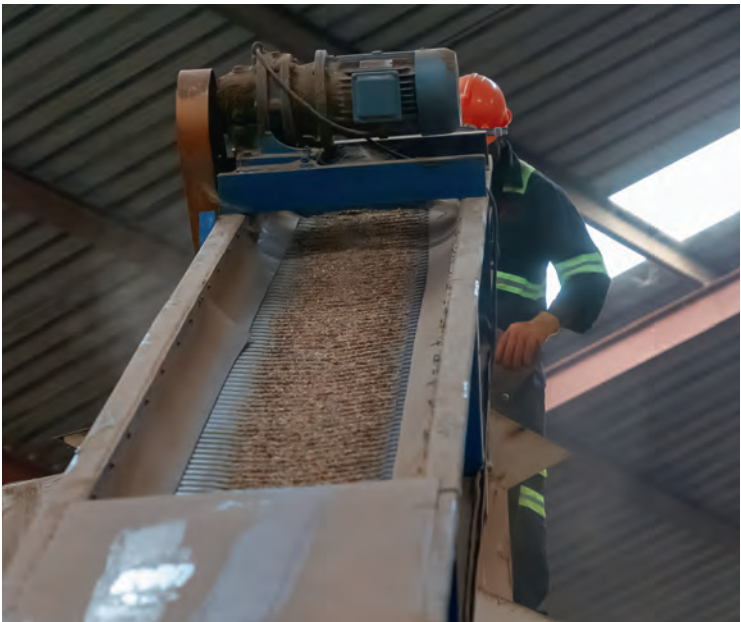
The dried feedstock en route to the pelletizer feed hopper.
