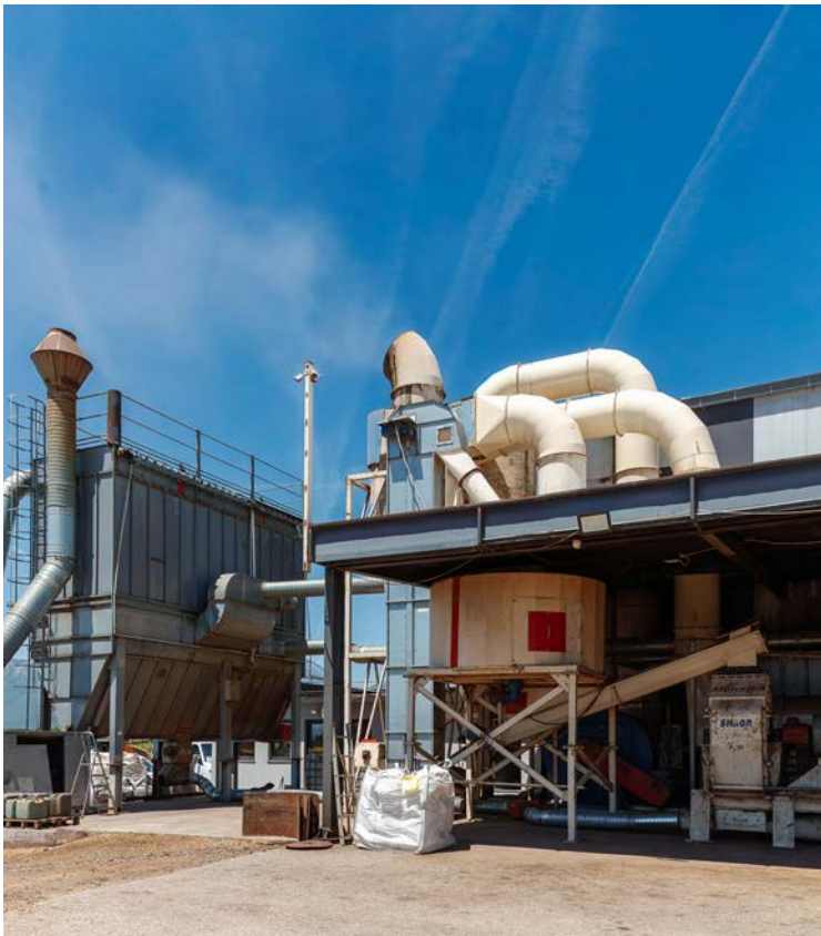
(Left) Pellets hot off the press heading for the cooler. (Above) A postcard view of the H&D Pellet facility. (Below left) The dryer cyclone, dust filter and flue exhaust. (Below right top) View of the woodyard with boiler fuel (left), the trailer chassis mounted Jenz HEM 582 chipper, and woodchips. (Below right below) Close-up of the dryer discharge, and dry grinder. (Bottom right) The two pelletisers, counterflow cooler and maturation silo. (Bottom centre) The Essegi F1000 automated weighing and bagging unit. (Bottom left) The automated Rendering Technologies palletising and wrapping unit.
