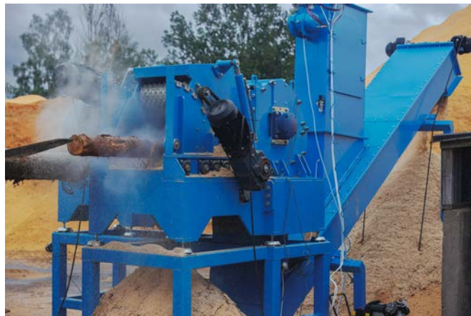
A woodyard demonstration of a KlingMill grinder awaiting installation at a wood pellet plant.
