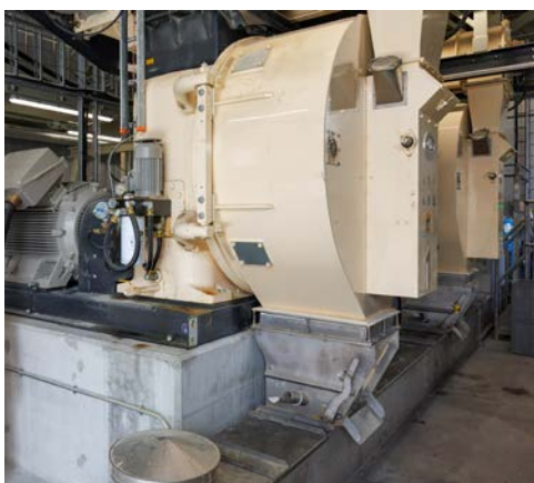
Two CPM presses with Twin-Track configurations.
