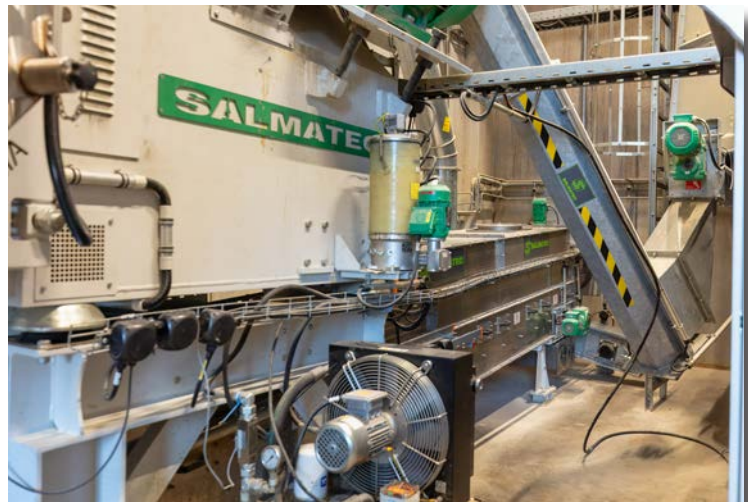
The pellets are cooled and sieved in a Salmatec-Rematec combined cooling sieve and discharge with the fines recirculated back to the press.
