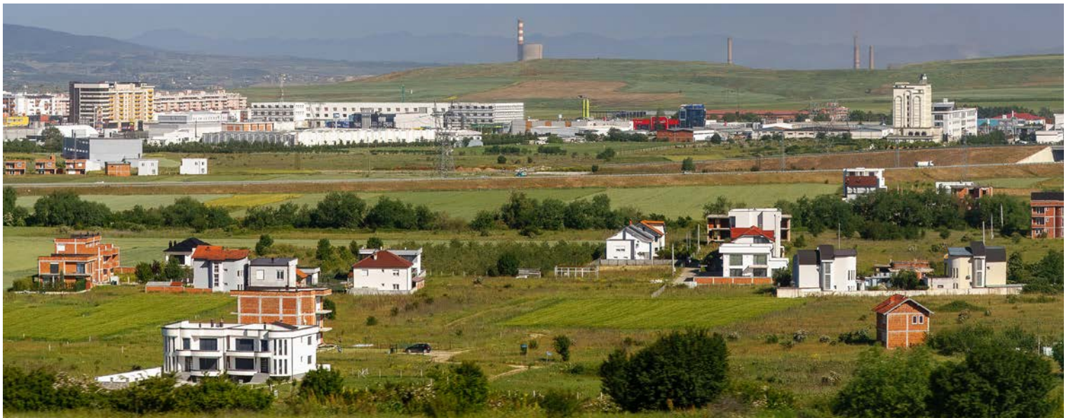
(Left) A memorial installation in central Prishtina. (Above) Western outskirts of Prishtina with the Kosova B and Kosova A lignite-fired power plants on the horizon – centre and right respectively. Comprising two 339 MW units, Kosova B was fully commissioned in 1984 and fully operational. The older Kosova A" consists of five units; A1 (65 MW) commissioned in 1962, A2 (125 MW) commissioned in 1965, A3 (200 MW) commissioned in 1970, A4 (200 MW) commissioned in 1971, and A5 (210 MW) commissioned in 1975. According to the current plan, units A3, A4 and A5 are operational, two are used in production, while one of them is a "hot" reserve due to their low readiness, which is a consequence of their age. Units A1 and A2 are out of service, without a defined status, (Top right) Fuelwood logs at a firewood producer. (Centre right) Air-dried boards in the woodyard of a furniture manufacturer. (Below right) Furniture production generates residues in the form of sawdust and off-cuts.
