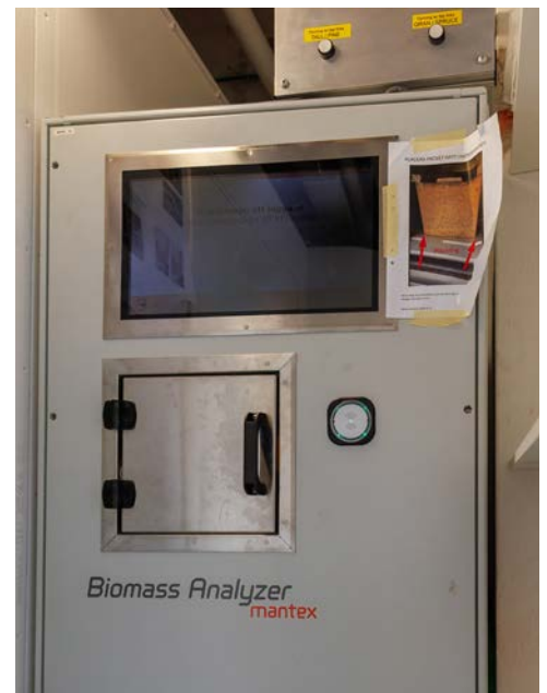
A first at a pellet plant, the Mantex Biomass Analyzer is an X-ray based method for measuring moisture content of incoming feedstock samples, and conducted by the driver as part of the delivery process.
